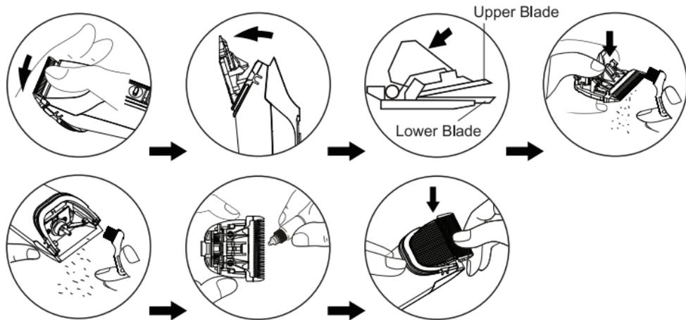
1. Before unloading the blade, make sure you have shut it down and separated the power line and the clipper.
